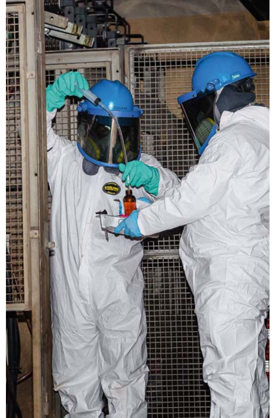
↑ Collecting an oil sample at an electrical substation. ← Technician Eva Huamani puts on a suit to protect her from electrical shocks.
