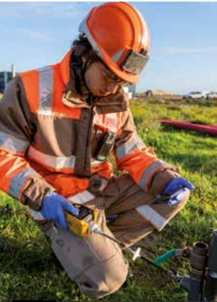
FRANCE - At the Dunkirk refinery decontamination site , a Colas Environnement employee takes readings to measure the pollutants present in the soil.
